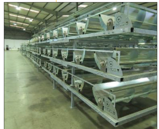
▲ Figure 10. MCG's CPC collectors with evacuated tube receiver.
