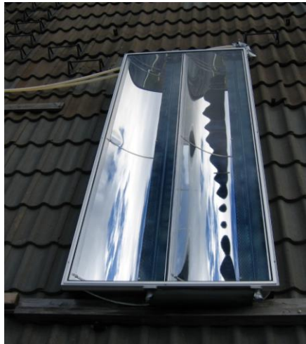
Figure 4 The CPC collector's transverse IAM measured with collector in vertical orientation (N-S)
