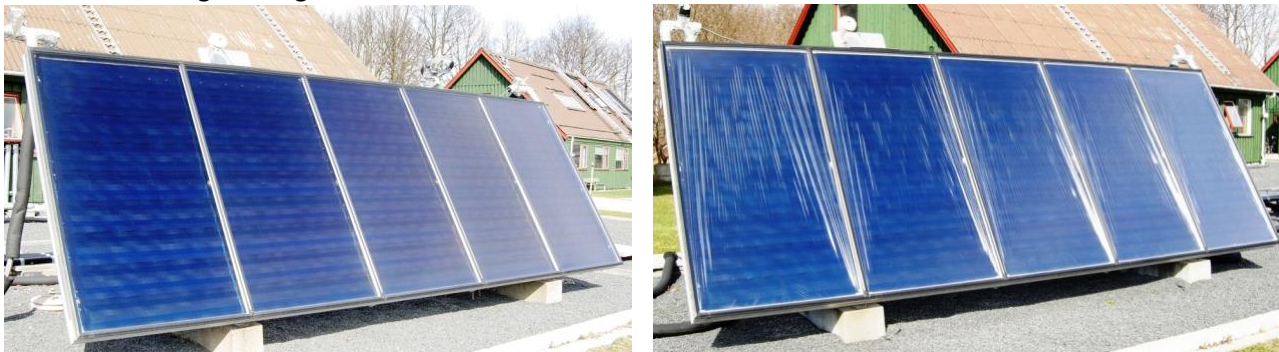
Figure 3.1: Solar collector HT-A 35-10 (left) and HT-SA 35-10 (right) at the Department of Civil Engineering at the Technical University of Denmark.
