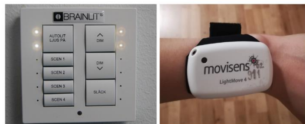
Figure 4. Left: one of the monitored offices. Top-right: overview of the scenes ( E_h stands for horizontal illuminance). Bottom-right: the manual switch to override the "lighting recipe" and the wrist-worn light logger used by the four employees.
