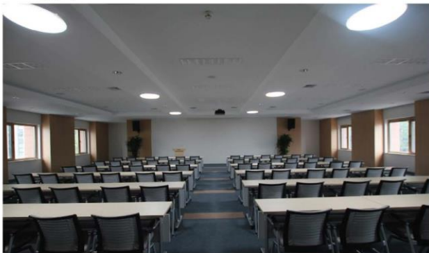
Figure 5. The CABR conference rooms. On the ceiling, the tubular daylighting system can be seen.
