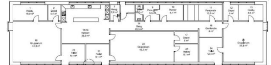
Floor plan. Total heated area is 330.4 m 2
